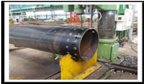
Fig 6.10 job is rotated &amp; locked with the pitch lock pin
