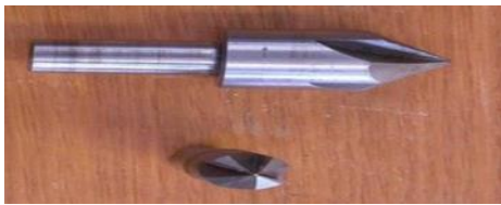
Fig 4.8 Counter sinking process and tool
